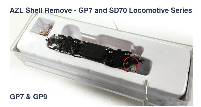
Step 1: Turn over locomotive. Turn the front truck slightly. Look for slight gap between the front of the metal chassis and the back of the plastic shell. This area is shown circled in red.
