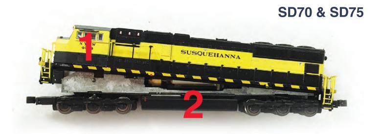
With your fore finger and thumb, hold both sides of the cab shell shown at point 1. With fore finger and thumb of the opposite hand, hold the chassis as shown at point 2, the fuel tank. Gently wiggle and lift up on the cab to loosen the shell. Once loose, the shell should be angled as shown. Now work the shell off while keeping the shell angle at a minimum to avoid bending the rear coupler. DO NOT hold or pull down on the trucks as they will separate and could be damaged.
