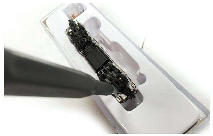
Step 2: Insert small flat head screw driver into gap. While holding the the locomotive, pull back on the screw driver. This will cause the front of the shell to separate from the chassis.
