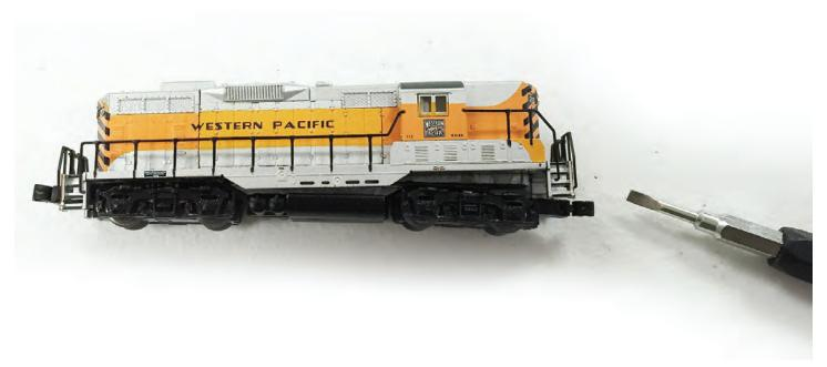
Step 3: With the front of the shell lifted, you can now gently pull of the shell. Try to lift up evenly has too sharp of an angle may cause the rear coupler to be pushed down.
